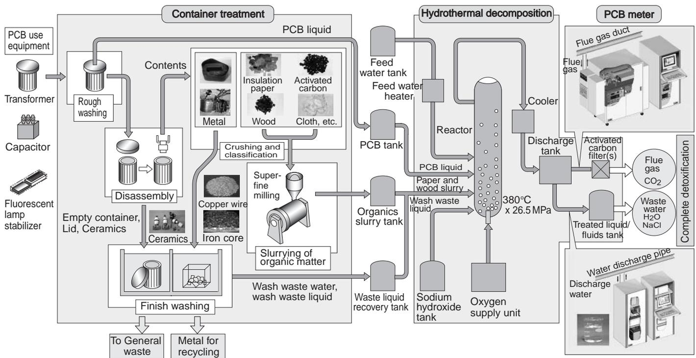
Fig. 4 PCB treatment flow Integrated PCB treatment flow including container, etc.
