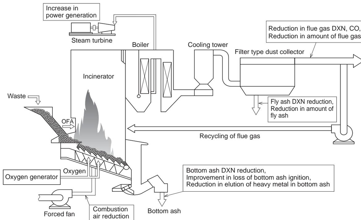
**Fig. 5 Next generation stoker type oxygen-enriched combustion system**
