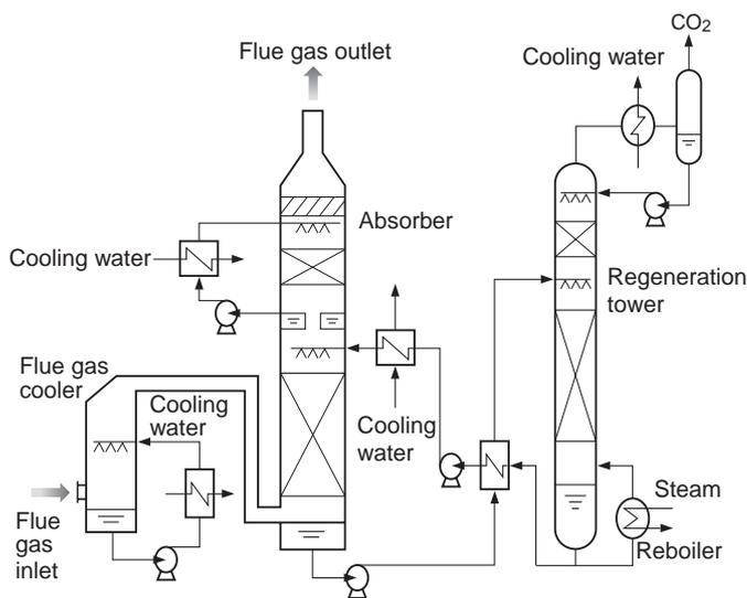
**Fig. 2 CO<sub>2</sub> Recovery facility**
