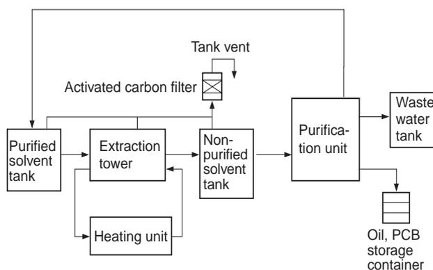
**Fig. 3 PCB contaminated soil remediation facility**
