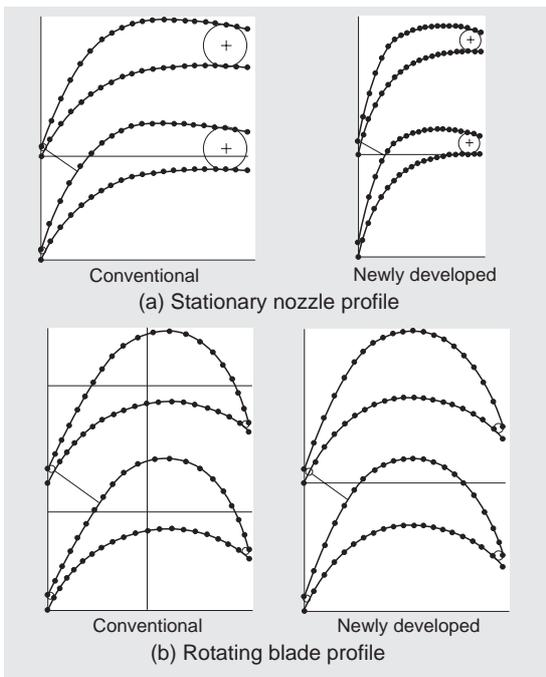
Fig. 8 Comparison of profiles between newly developed type and conventional type
