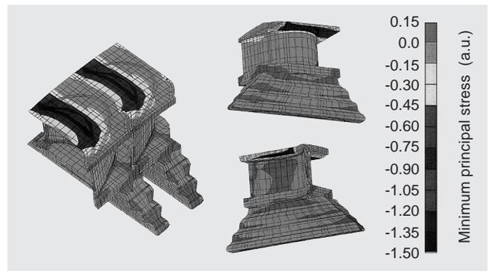
**Fig. 3 Results of FEM analysis (minimum principal stress distribution)**
