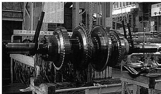
**Fig. 4 Assembled test rotor of parallel short ISB**
