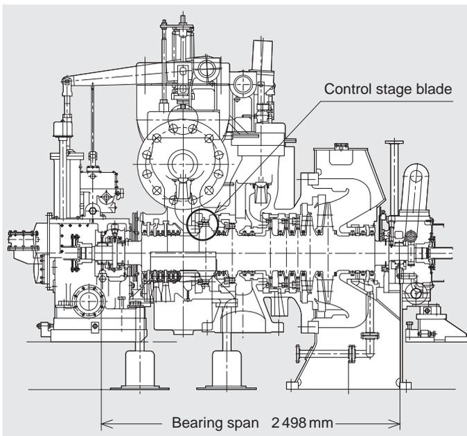
Fig. 1 Cross-sectional view of SYN. GAS turbine
