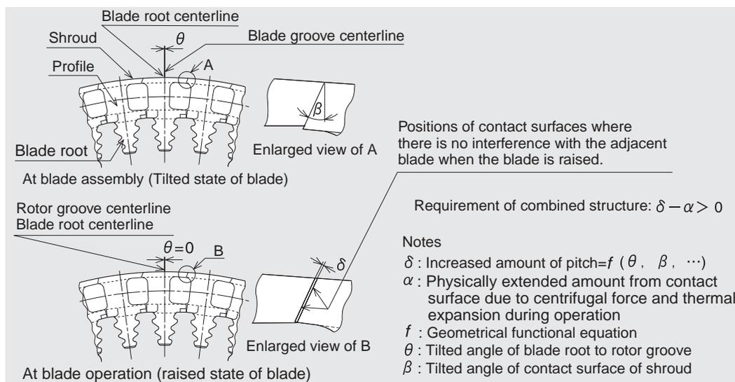
Fig. 2 Combined structure of parallel short ISB
