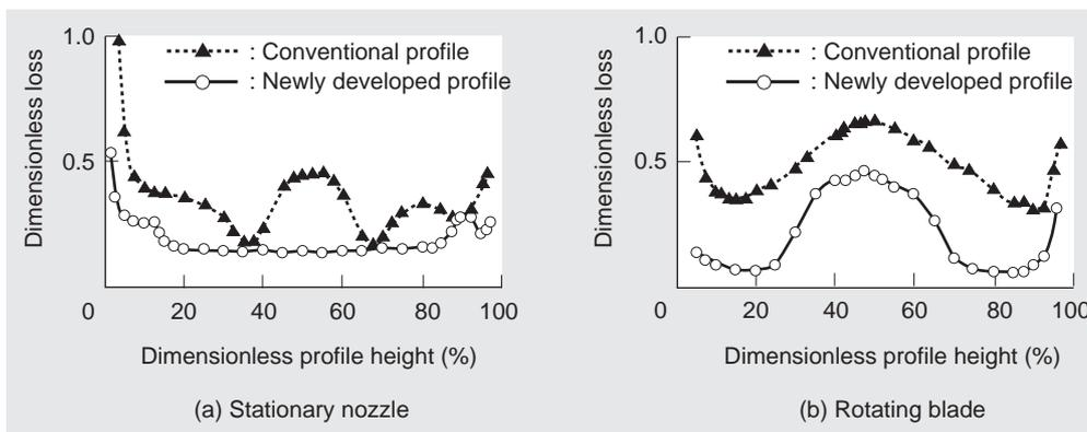
Fig. 10 Results of cascade test
