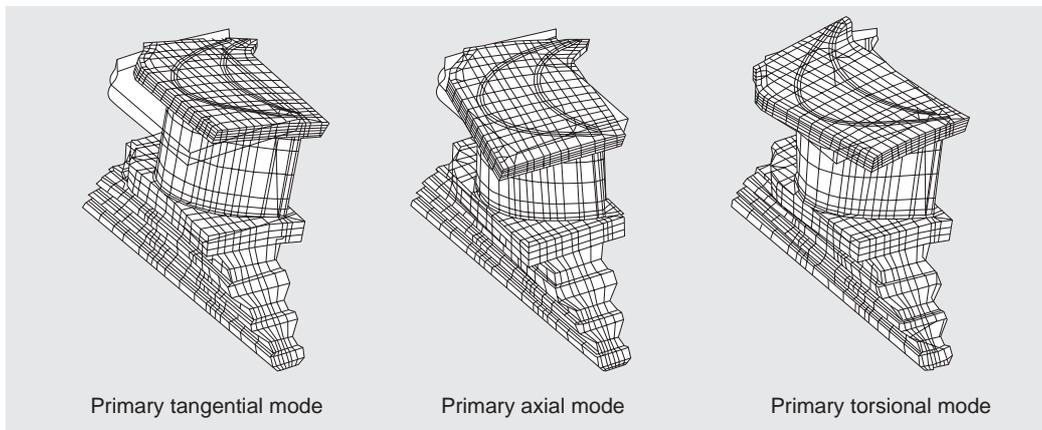
Fig. 6 Results of calculated mode shapes of minimum order in different directions
