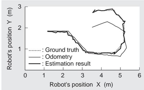
Fig. 3 Example of self-localization
