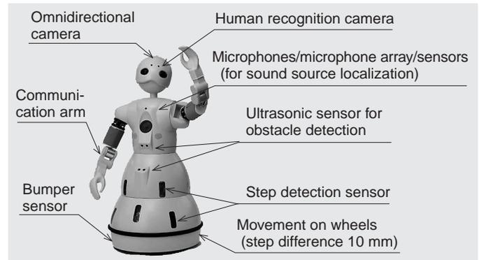
Fig. 1 Configuration of home-use robot "wakamaru"
