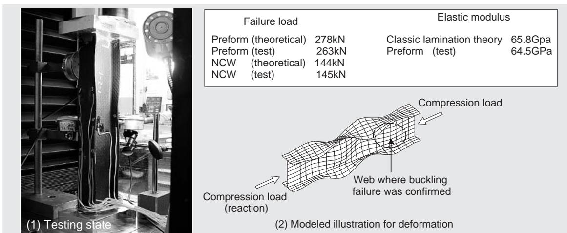
**Fig. 9** Compression test for stringer unit The test values and theoretical values for the NCW fabric were in agreement, but in the case of the preform, both of strength and elastic modulus were lower than the tested value.
