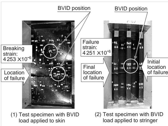
**Fig. 8 Compression test result of test specimen applied BVID**
