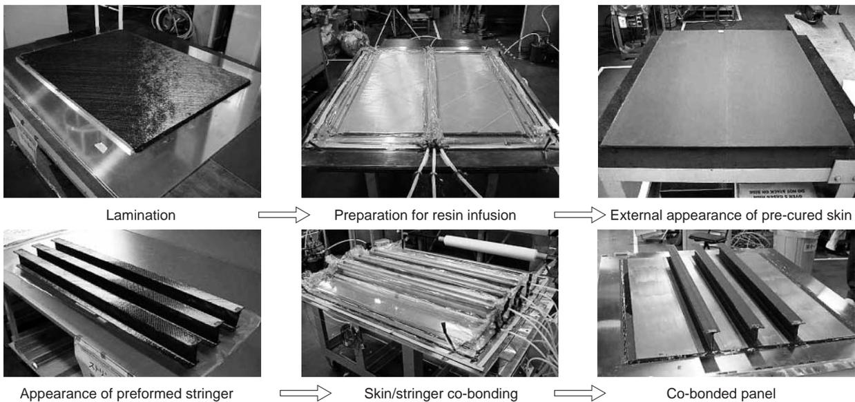
Fig. 5 Fabrication process of three stringers panel
