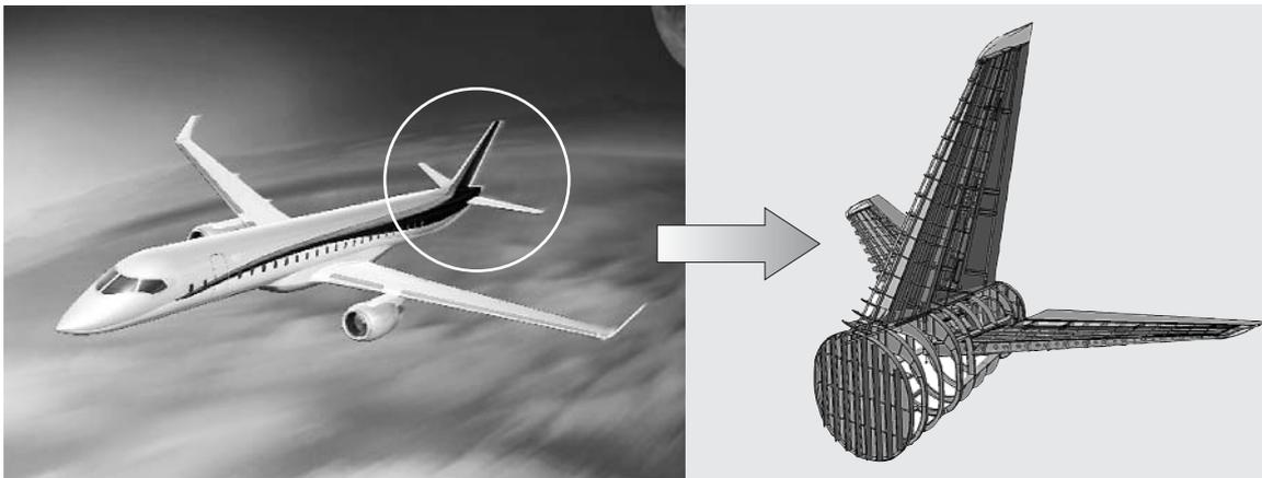
**Fig. 1 Empennage structure of Mitsubishi Jet**
