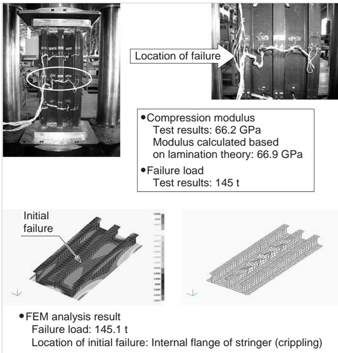
**Fig. 7 Compression test for three-stringer panel**
