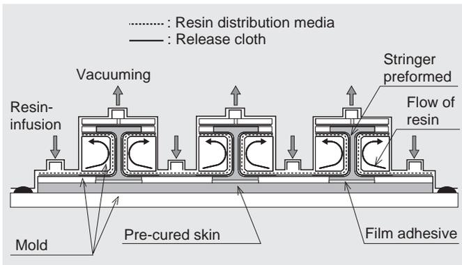
**Fig. 6 Set up of skin/stringer co-bonding process**
