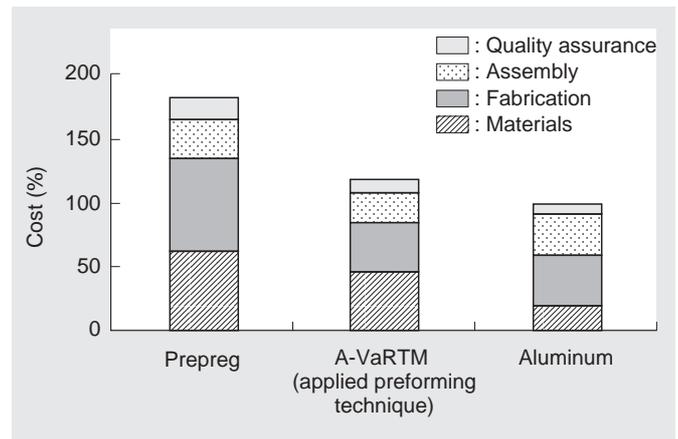
**Fig. 10 Comparison of costs for empennage box structure**
