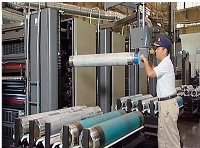
Fig. 2 Sleeve exchange operation
