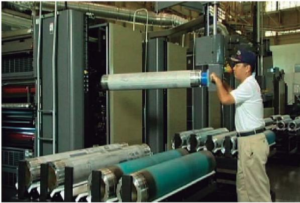
Fig. 2 Sleeve exchange operation
