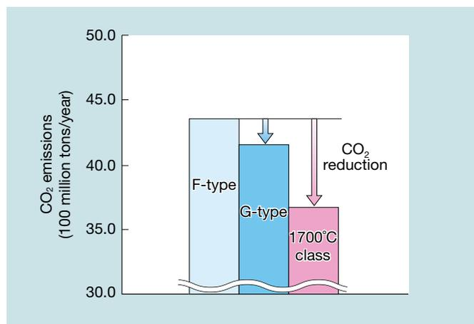
**Fig. 7 Estimated CO<sub>2</sub> emissions due to power generation at natural gas firing combined cycle plant**
