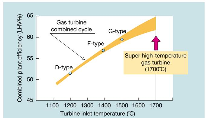
**Fig. 4 Turbine inlet temperature and combined plant efficiency**
