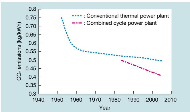
**Fig. 3 Transition of “CO<sub>2</sub> emission reduction”**
