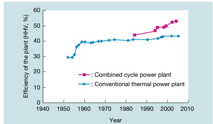
**Fig. 2 Transition of plant efficiency of conventional type thermal power plant and combined cycle power plant :**
