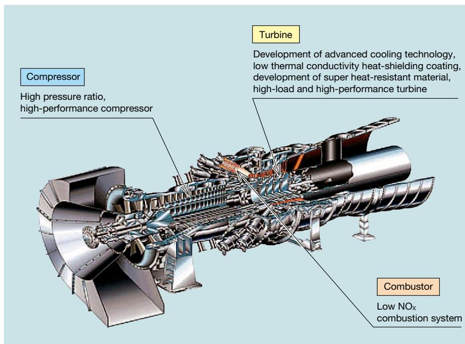
**Fig. 5 Design concept of 1,700°C class gas turbine**
