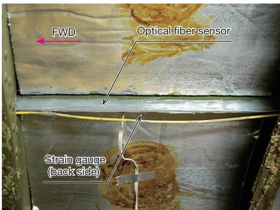
**Fig. 6 The installed optical fiber**
