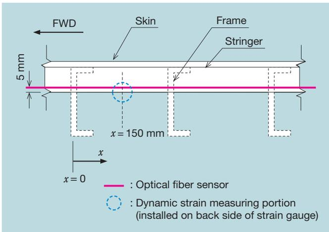
**Fig. 5 Schematic view of the optical fiber installation**
