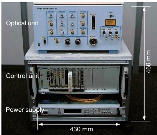
Fig. 2 The onboard BOCDA device
