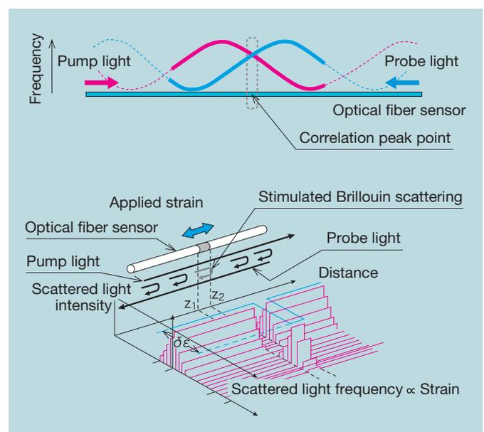
Fig. 1 BOCDA measurement principles
