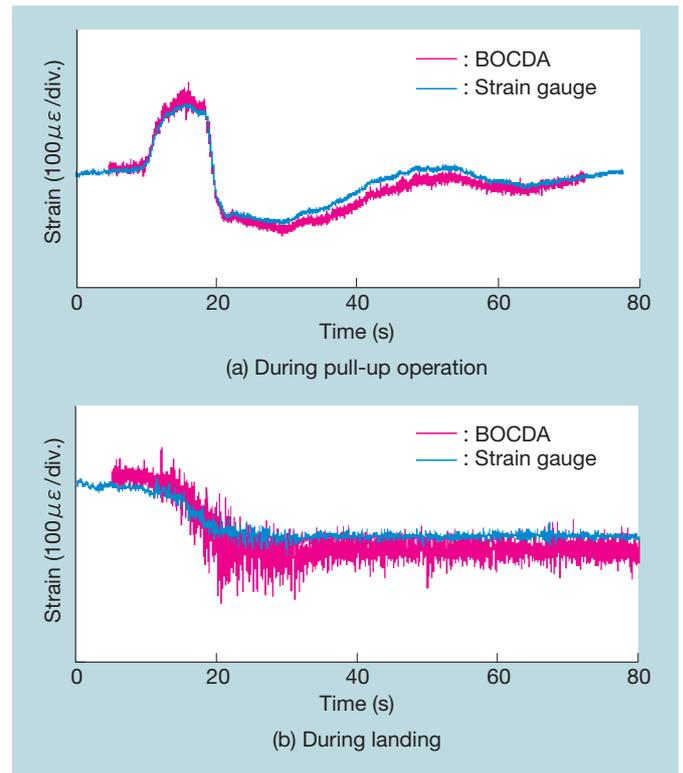
**Fig. 7 The strain history in the fuselage panel measured using the BOCDA device**
