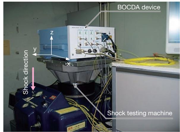
Fig. 3 The shock test of the BOCDA system
