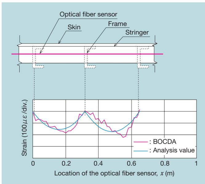
**Fig. 8 BOCDA measurement of the fuselage panel distributed strain**
