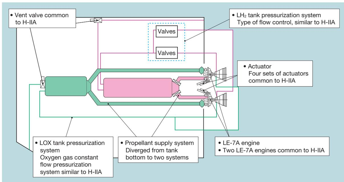
Fig. 5 Overview of the first-stage propulsion system
