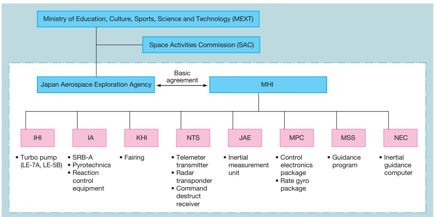
**Fig. 2 H-IIB launch vehicle development framework**
