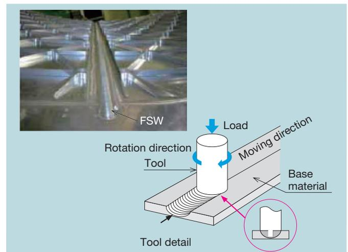
**Fig. 3 Conceptual diagram of FSW**
