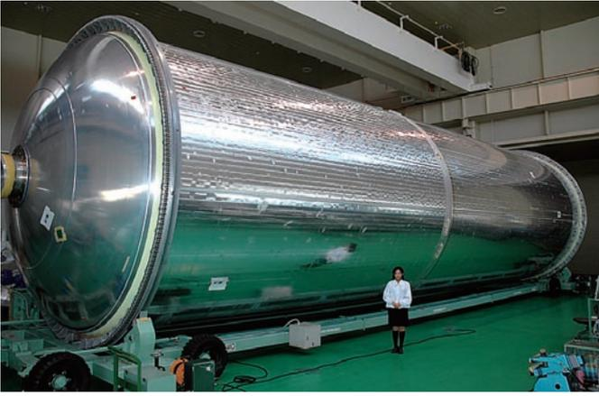
Fig. 4 LH<sub>2</sub> tank for the test flight (diameter: 5.2 m, length: 19.4 m)
