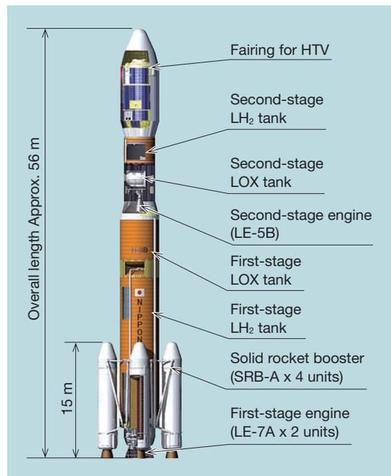
**Fig. 1 Overview of the H-IIB launch vehicle**
