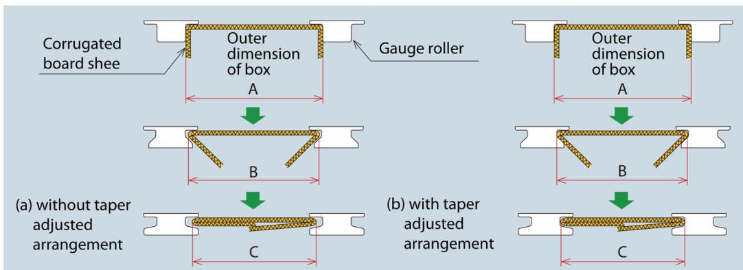
**Figure 4 Schematic of taper adjusted arrangement for gauging roller (cross section showing the traveling direction of the sheet)**
