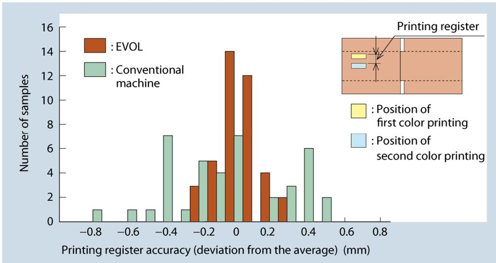
**Figure 3 Example of printing register accuracy (comparison with data of conventional type)**
