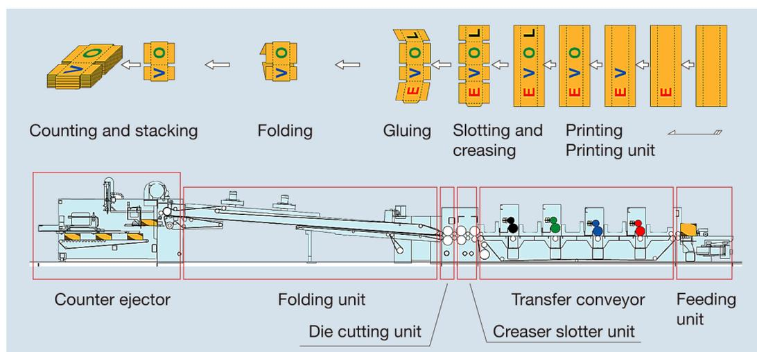
**Figure 1 Basic configuration of a corrugated board box making machine**
