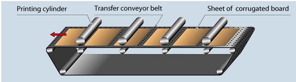
**Figure 2 One-piece belt-type transfer conveyor**
