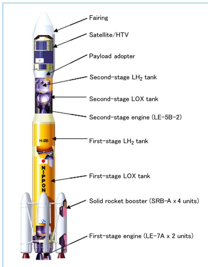
Figure 1 Overview of the H-IIB launch vehicle
