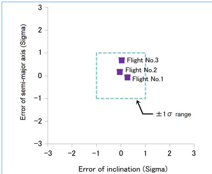
Figure 2 Orbit insertion accuracy
