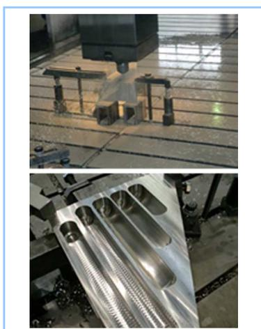
**Figure 5 Primary tests for RP grooving**
