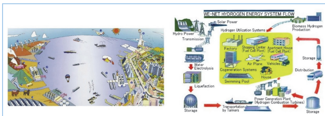
Figure 1 Schematic representation of WE-NET (5)
