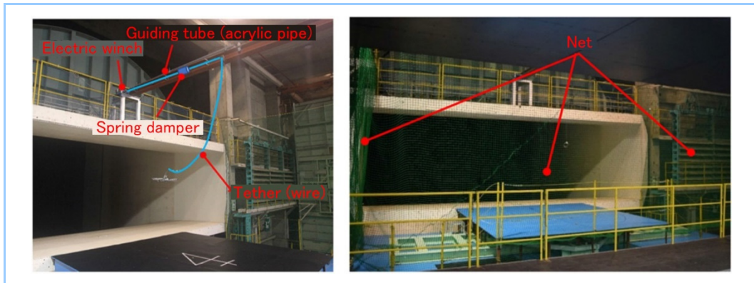
Figure 2 Safety devices (Left: Tether system, Right: Safety catch nets)
