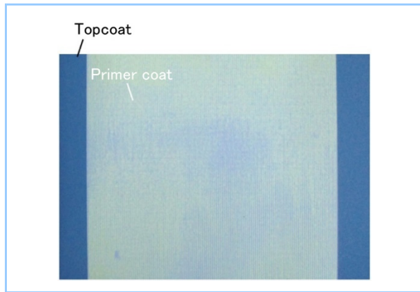
Figure 11 Appearance of test piece after paint stripping under combination of high-speed and selective removal conditions
